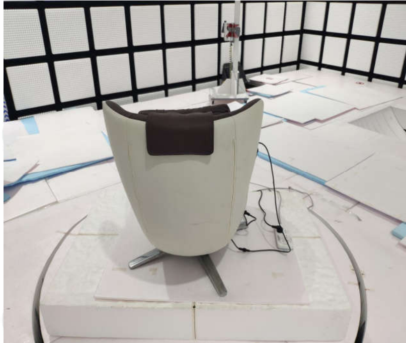
Radiated spurious emission Test Setup-3(Above 1GHz)
