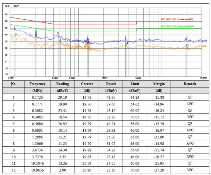
\*\*\*Note: 1). Pre-scan all modes and recorded the worst case results in this report BT LE (Middle Channel). 2). Result = Reading + Correct, Margin = Result – Limit.
