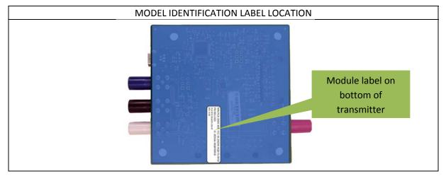
Module FCC ID: The transmitter model identification label contains the module's FCC ID number.
