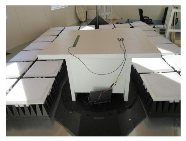
Radiated Above 1 GHz - Onboard Antenna
