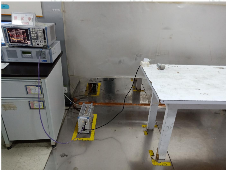
Conducted Emissions Test Setup
