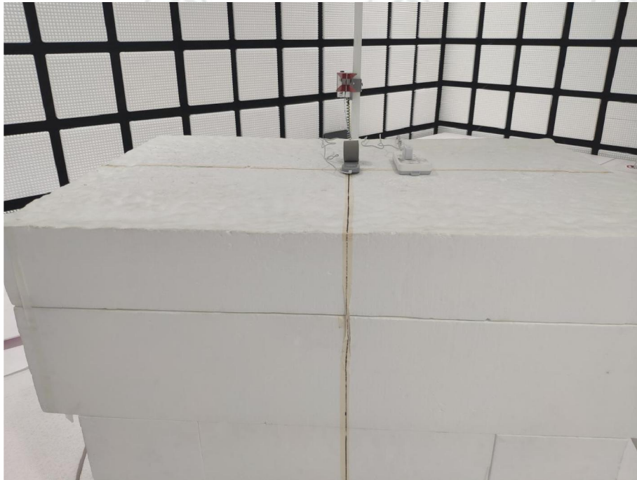
Radiated spurious emission Test Setup-2(Above 1GHz)
