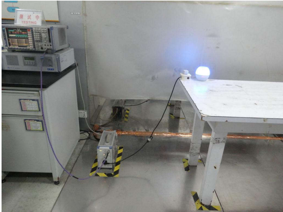
Conducted Emissions Test Setup
