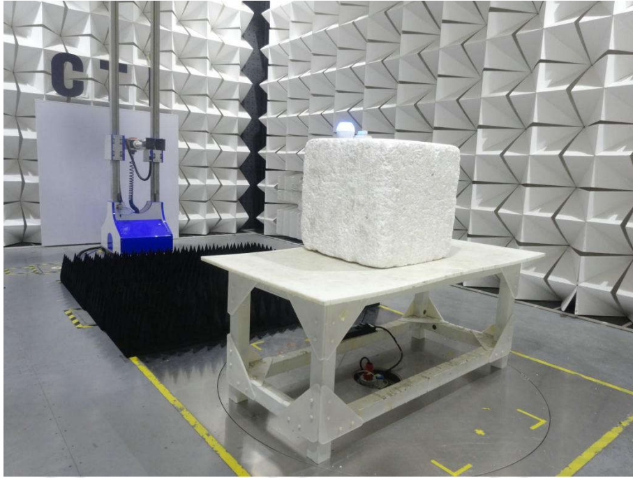
Radiated spurious emission Test Setup-3(Above 1GHz)
