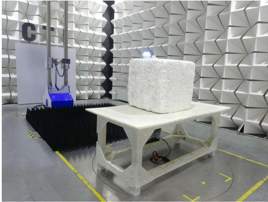
Radiated spurious emission Test Setup-3(Above 1GHz)
