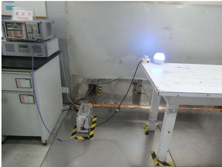
Conducted Emissions Test Setup
