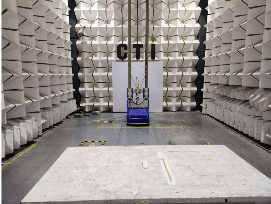
Radiated spurious emission Test Setup-1(Below 1GHz)
