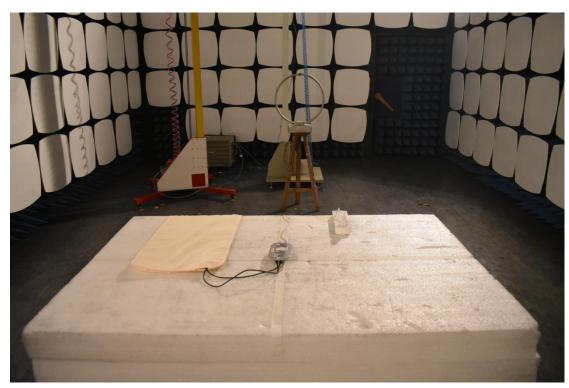
3. Radiated emission (9KHz-30MHz)
