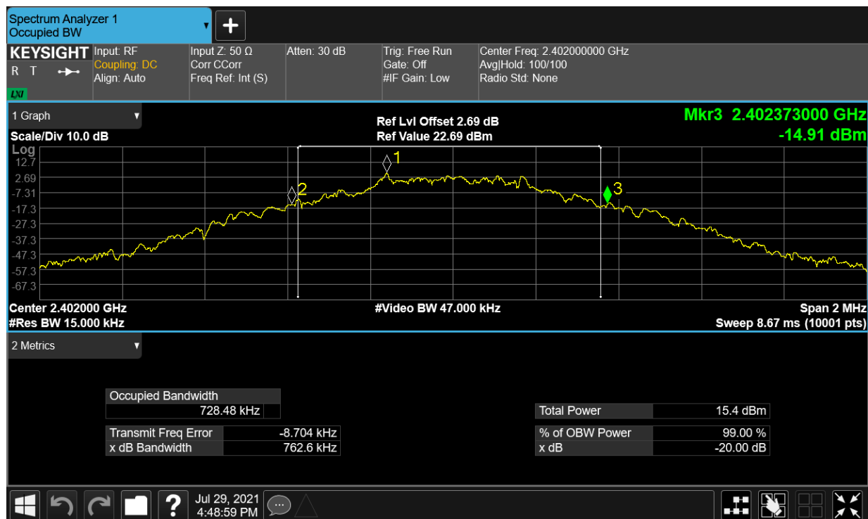
-20dB Bandwidth NVNT 1-DH1 2441MHz Ant1
