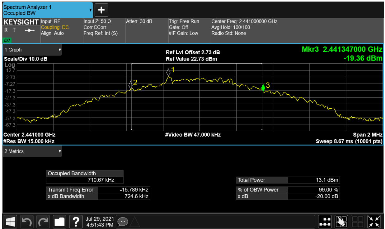
-20dB Bandwidth NVNT 1-DH1 2480MHz Ant1
