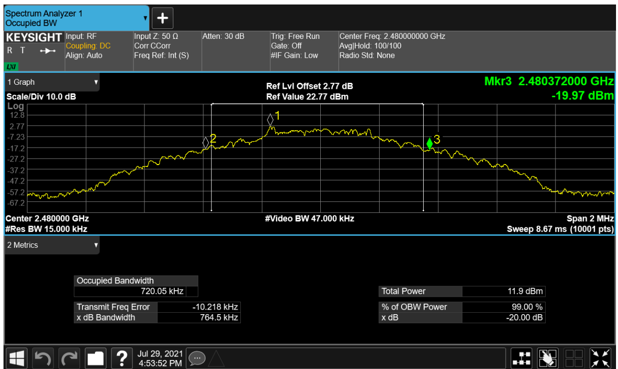
-20dB Bandwidth NVNT 2-DH1 2402MHz Ant1
