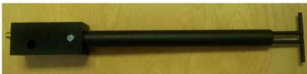
Figure 1 – MVG COMOSAR Validation Dipole
