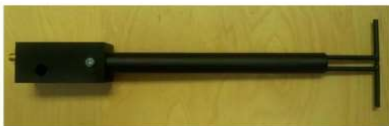
Figure 1 – MVG COMOSAR Validation Dipole
