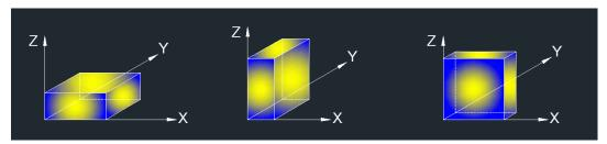
Note: The EUT was investigated in three orthogonal orientations X/Y/Z on ANT0 to determine the worst-case orientation. X orientation is finally determined the worst.
