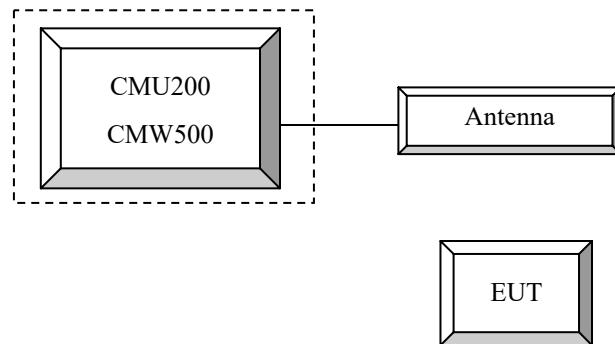
**Block Diagram of Test Setup**
