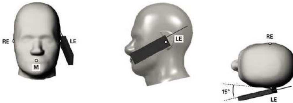
Fig.11.4 Illustration for Tilted Position
