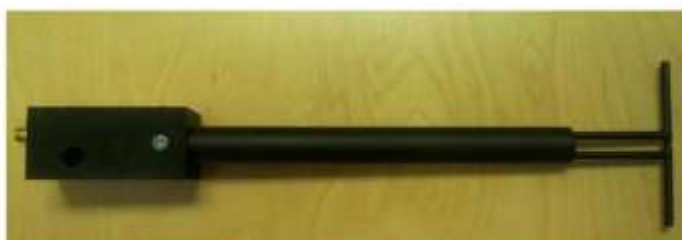
Figure 1 – MVG COMOSAR Validation Dipole
