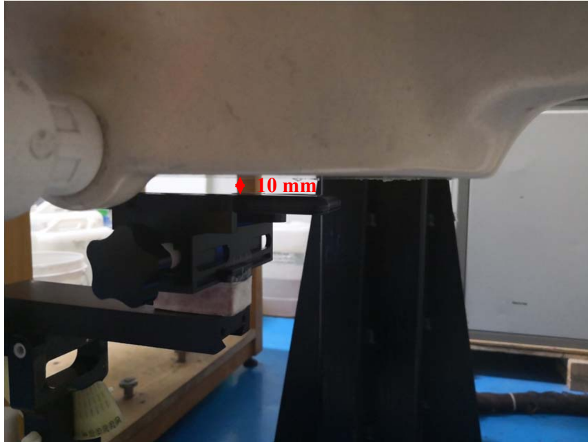
Body (Worn) Back Setup Photo (10mm)
