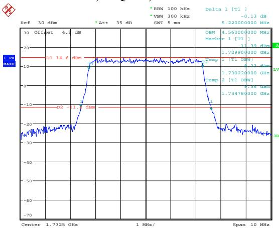
**5M, QPSK, High Channel**
