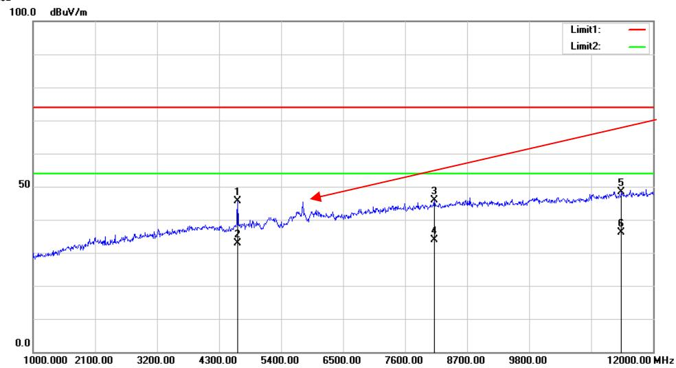
Fundamental Test with Band Rejection Filter
