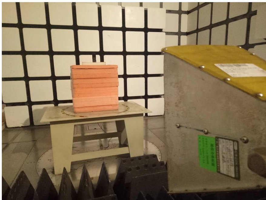
Radiated Emissions View (Above 1 GHz)
