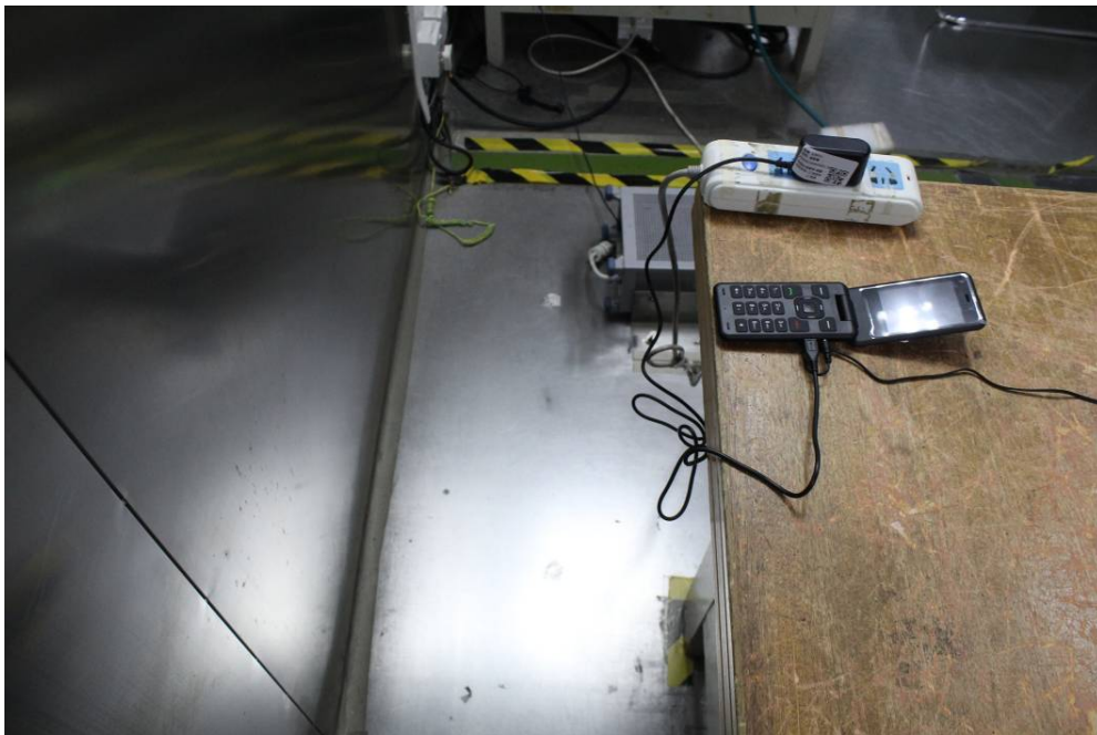
Conducted Emissions - Side View
