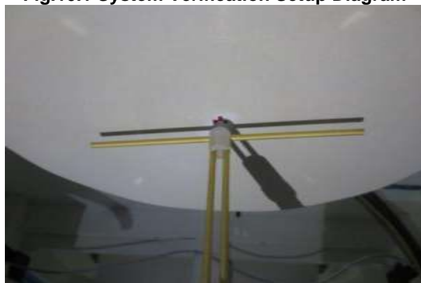
Fig.10.2 Photo of Dipole setup
