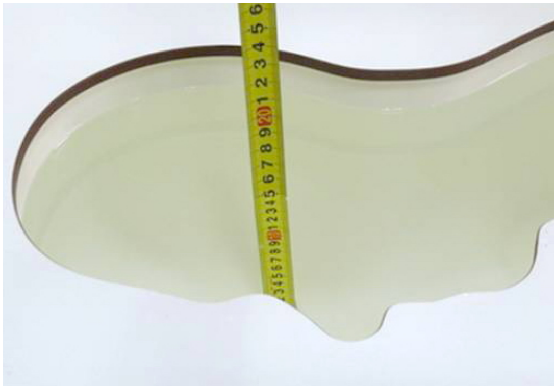
Liquid depth in the head Phantom (1750 MHz, 15.4cm depth)
