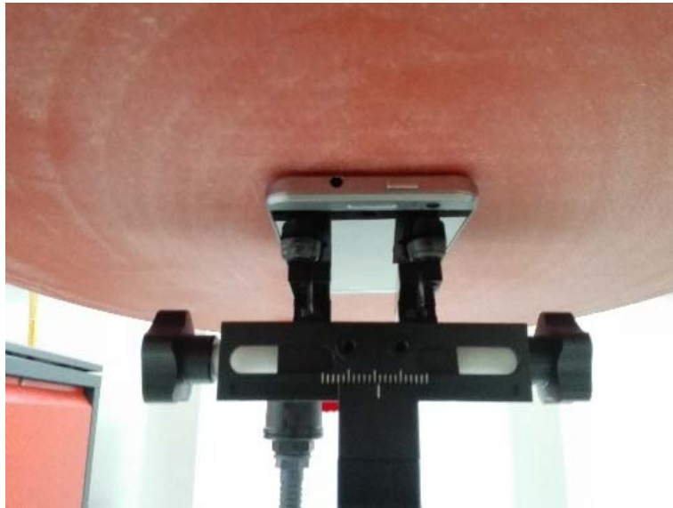
0mm Body-worn Rear Setup Photo
