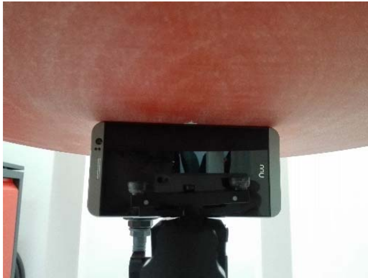
0mm Body-worn Right Side Setup Photo
