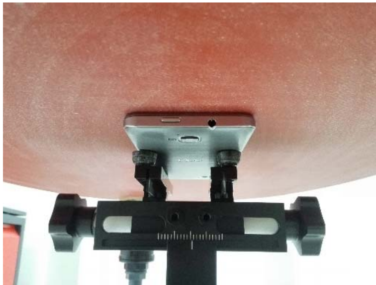
0mm Body-worn Rear Setup Photo
