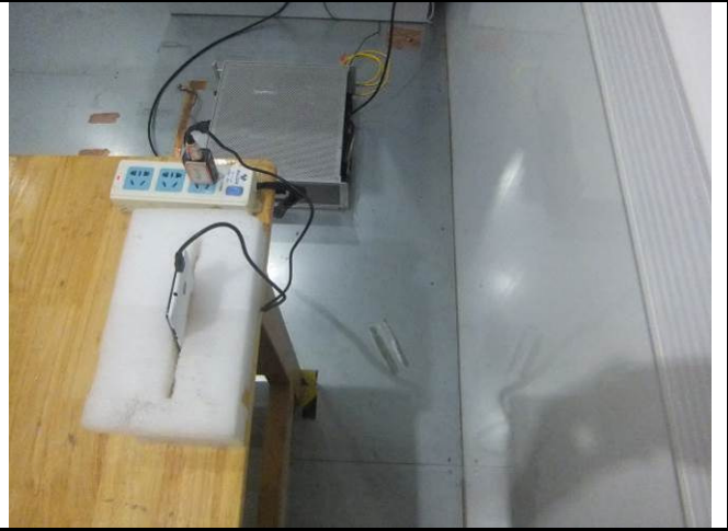
Conducted Emissions Test Setup Side View
