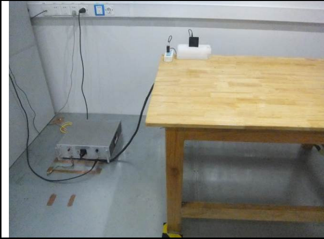
Conducted Emissions Test Setup Front View
