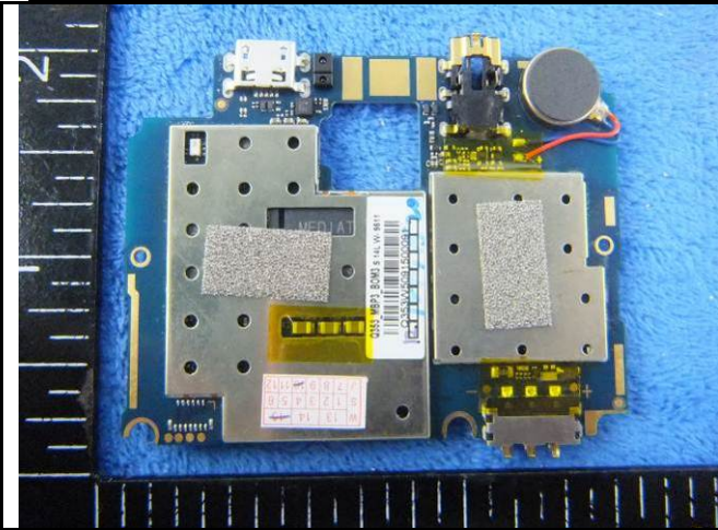
Mainboard with Shielding - Rear View
