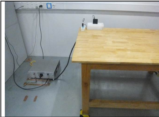
Conducted Emissions Test Setup Front View
