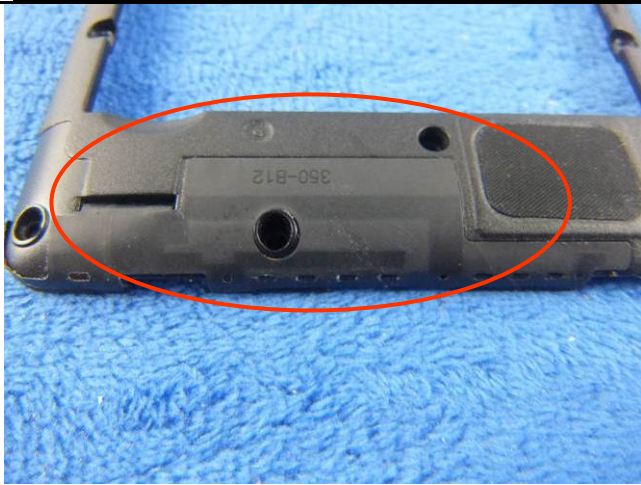
GSM/PCS/UMTS-FDD/LTE Antenna View
