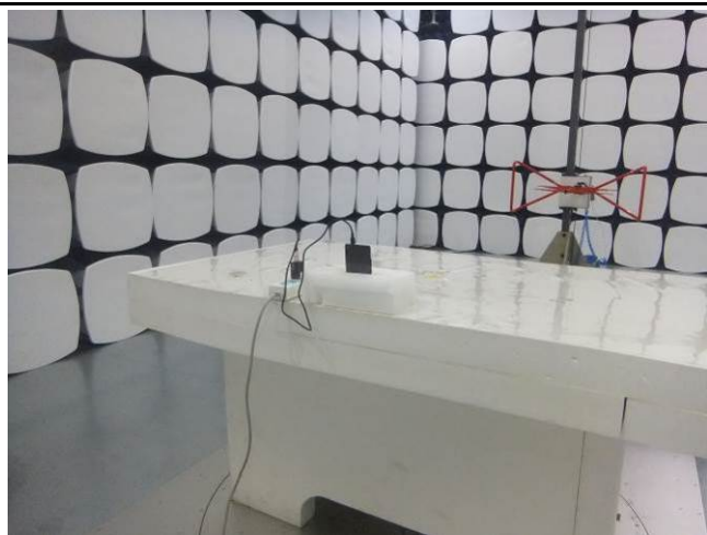
Conducted Emissions Test Setup Front View
