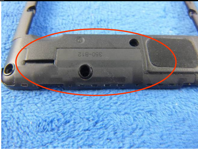
GSM/PCS/UMTS-FDD/LTE Antenna View
