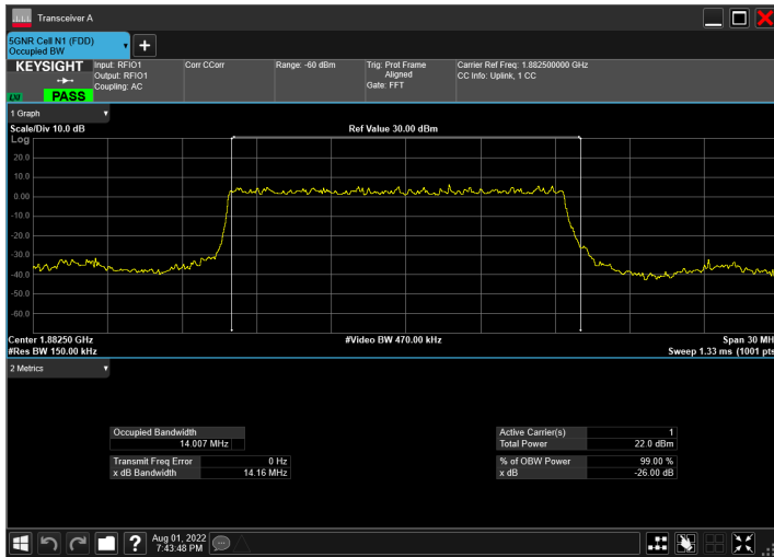
n25_15MHz_15kHz_1882.5MHz_DFT-s-OFDM PI/2 BPSK_RB75@0
