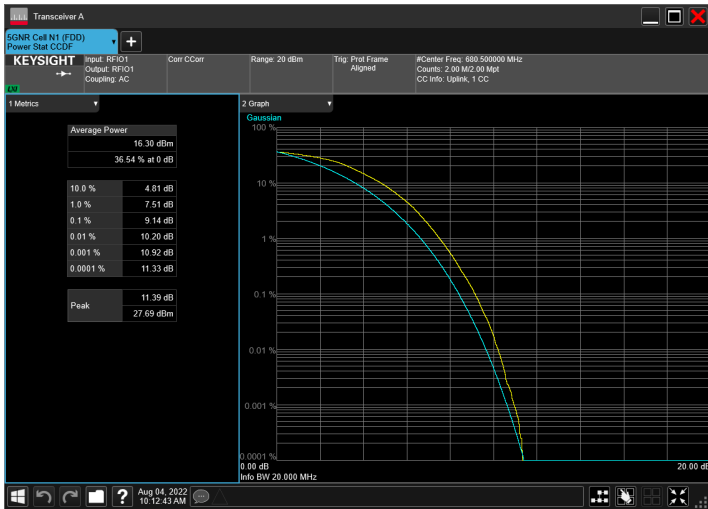
DC_2A_n71A_10MHz|20MHz_15kHz_1880MHz|680.5MHz_D FT-s-OFDM 64 QAM_RB0|RB100@0
