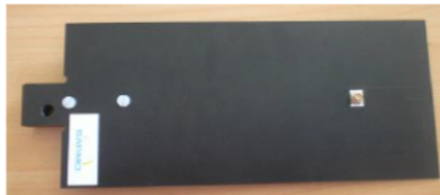
Figure 1 – MVG COMOHAC Validation Dipole
