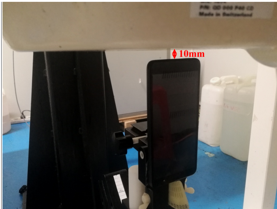
Body Bottom Setup Photo (10mm)
