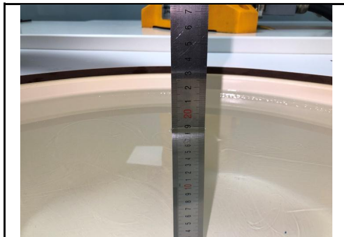
Fig. 9.8 Photo of Liquid Height for Body SAR (5200MHz~5800MHz) (depth>15cm)
