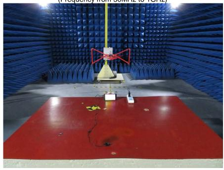
RADIATED EMISSION TEST (Frequency above 1GHz)
