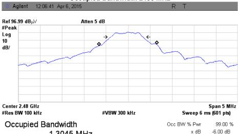
Transmit Freq Error -3.033 kHz x dB Bandwidth 722.238 kHz
