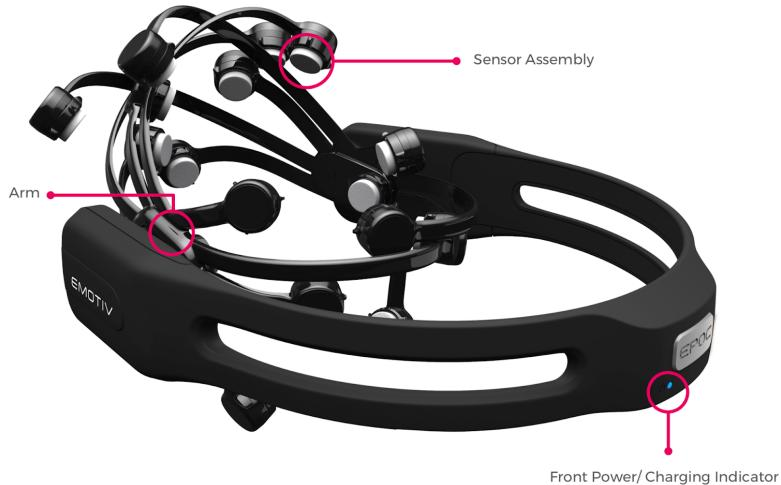
The EPOC X has two electrode arms each containing 9 locations (7 sensors + 2 references). Two sensor locations (M1 / M2) already have comfort pads fitted because they are the alternative positions for the default references (P3 / P4).
