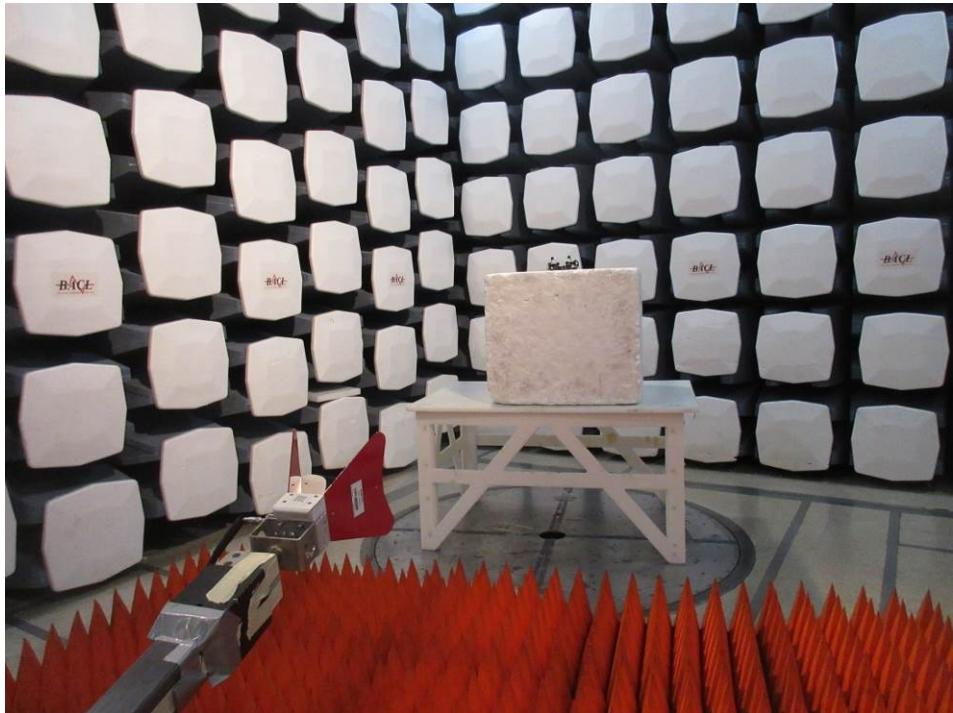
**Radiated Spurious Emissions Test: 1 – 18 GHz – 3 meters – Rear View**
