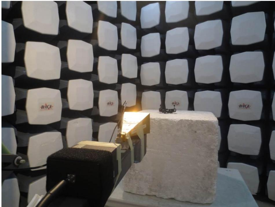
**Radiated Spurious Emissions Test: 18 – 26.5 GHz – 1 meter – Rear View**
