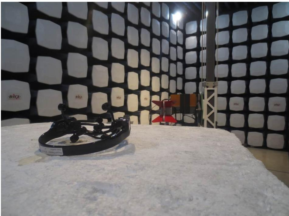
**Radiated Spurious Emissions Test: 18 – 26.5 GHz – 1 meter – Front View**
