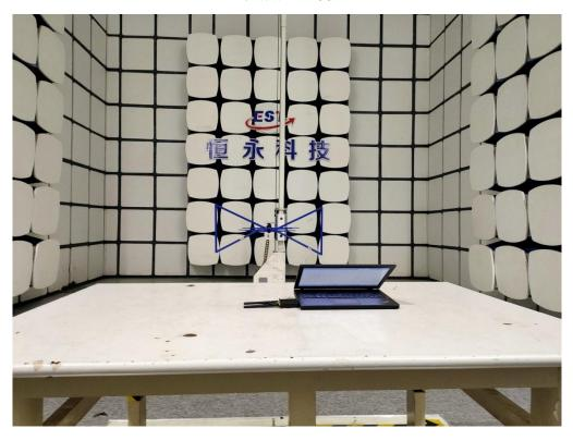
Radiated Test (Above 1GHz)
