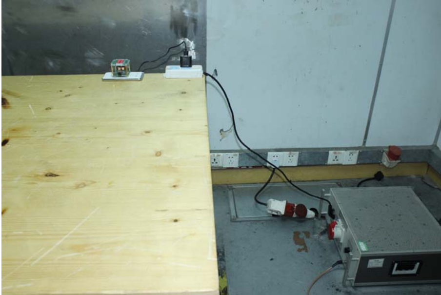
Photo of Power Line Conducted Emission Measurement
