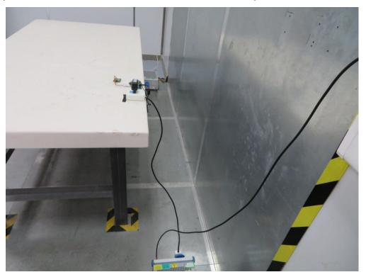
Description: Back View of the Conducted Emission Test Setup for  $0.15 MHz \sim 30 MHz$
