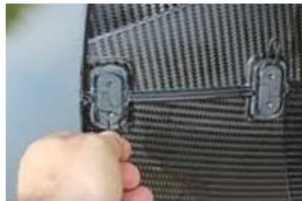
Figure 3-7: Latches to interconnect the four panels
