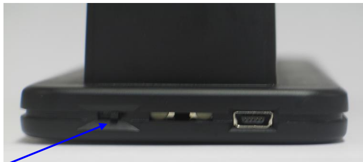
Figure 9: CaptiView Display On/Off Switch
