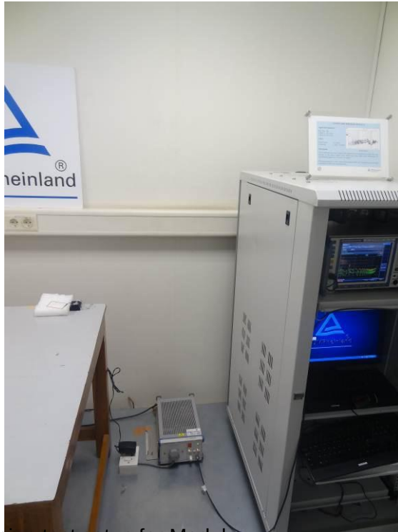
Conducted Emission test setup for Module
