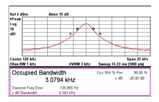
Test Plot: Centre Frequency 120 kHz
