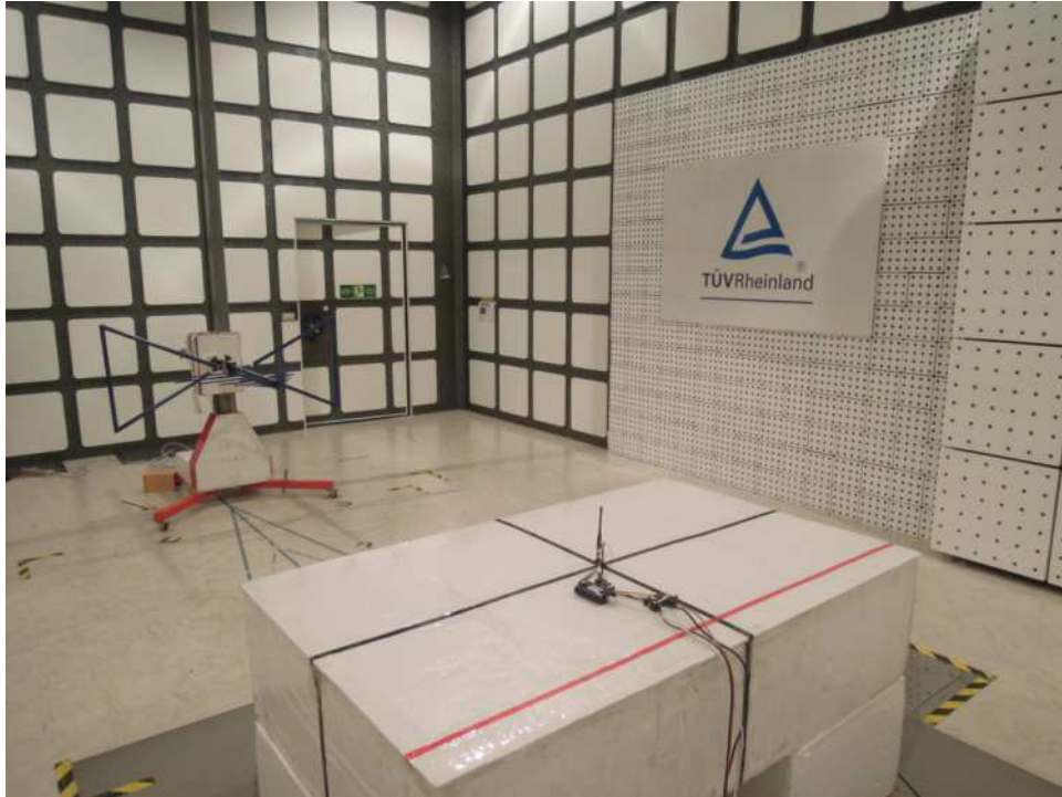
Photograph 3: Set-up for Spurious Emissions (Front View 2)- RFA-02-5-C7H1-ANT
