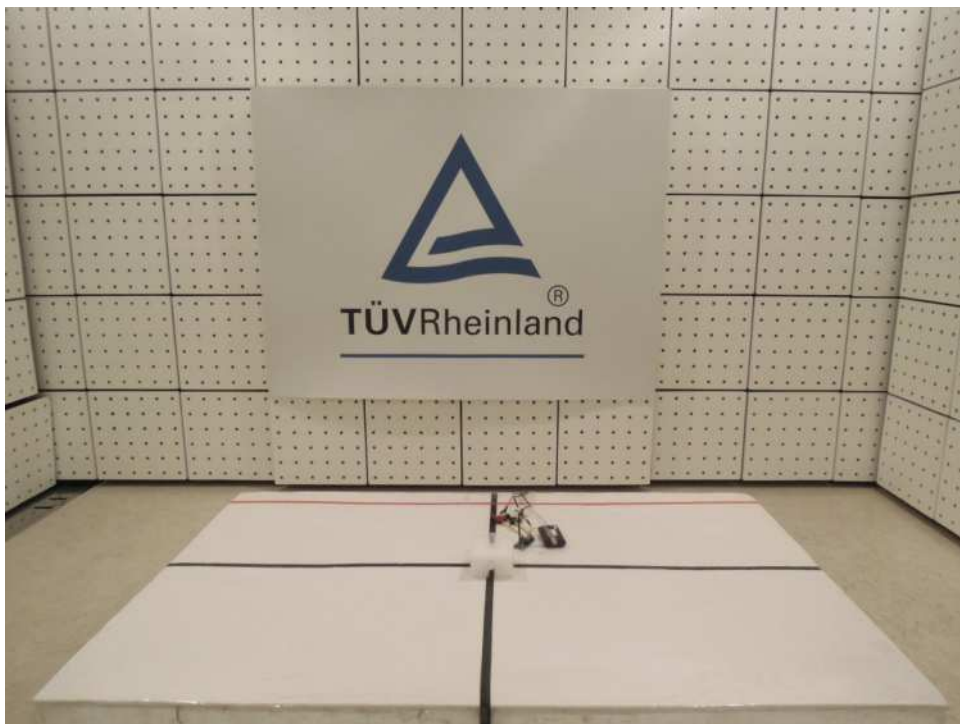
Photograph 7: Set-up for Spurious Emissions (Front View 1)- RFPCA381013IMAB701-ANT
