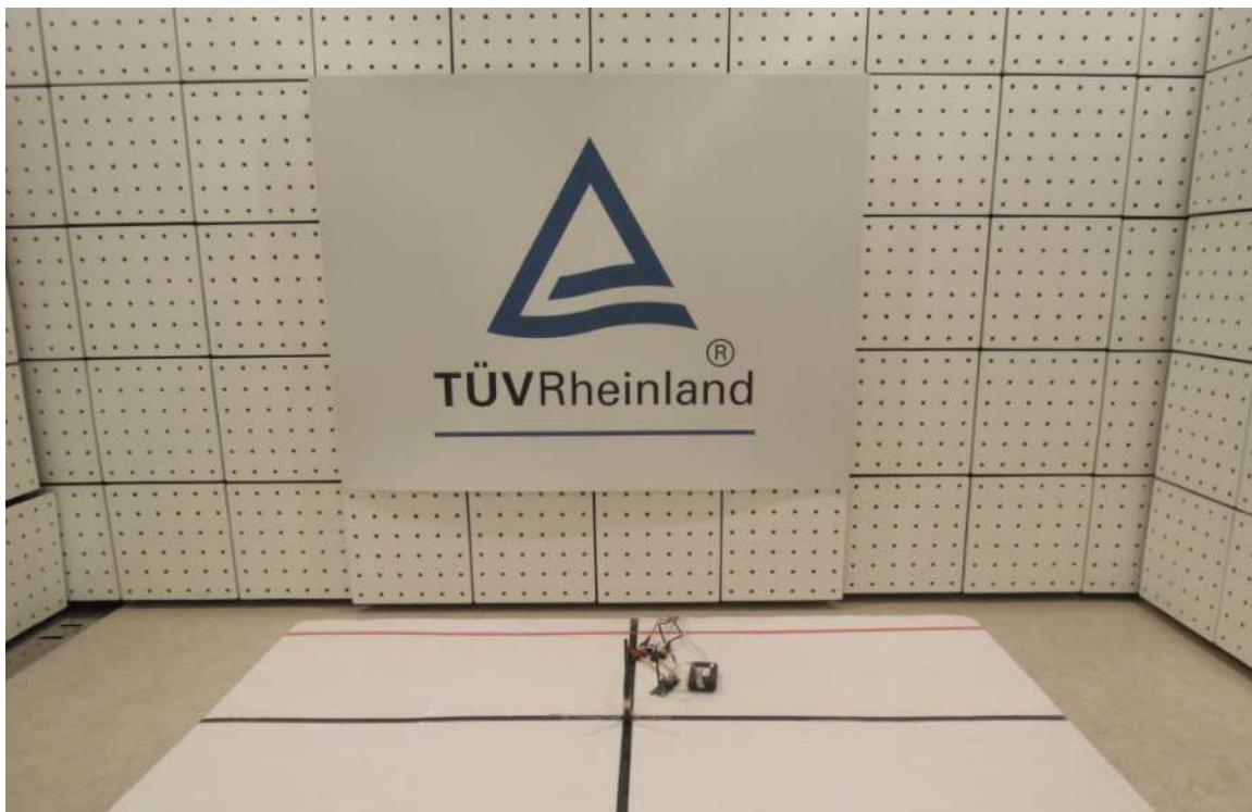
Photograph 1: Set-up for Spurious Emissions (Front View 1)- RFA-02-5-C7H1-ANT
