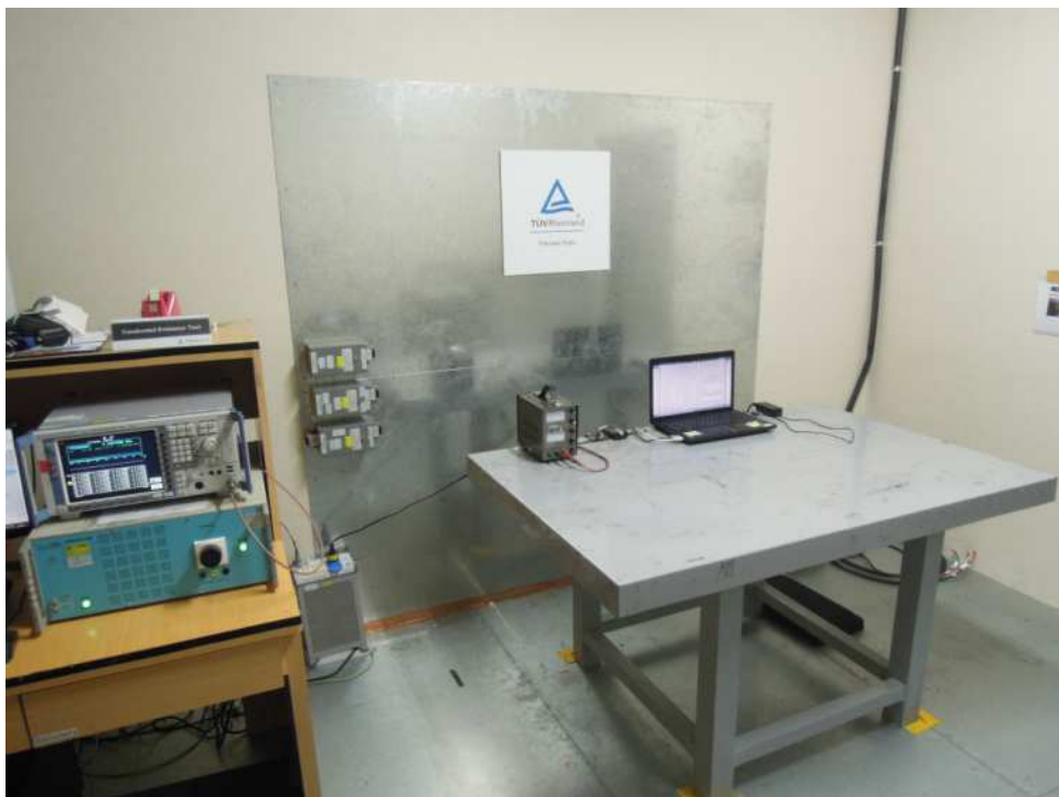
Photograph 27: Set-up for Mains Conducted testing (Front View)
