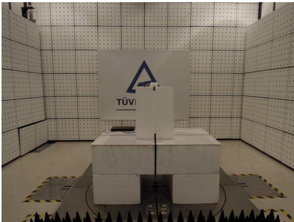
Photograph 21: Set-up for Spurious Emissions (Front View)- 1461530100 -ANT
