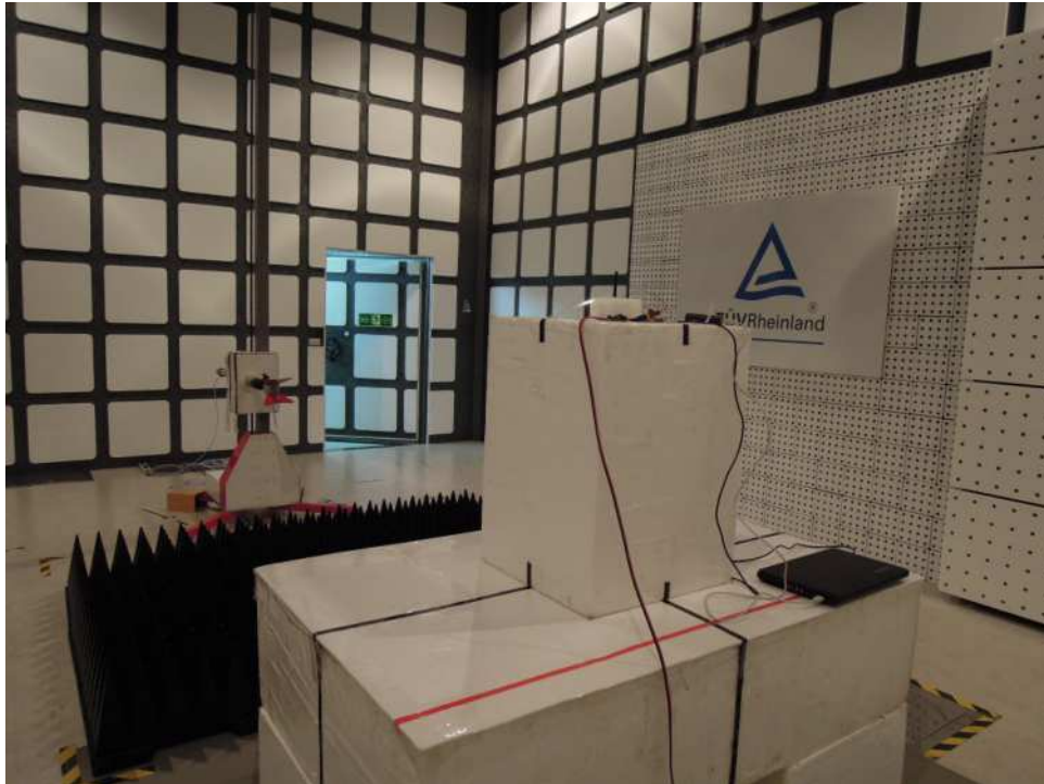
Photograph 19: Set-up for Spurious Emissions (Front View)- RFA-02-3-C5H1 -ANT
