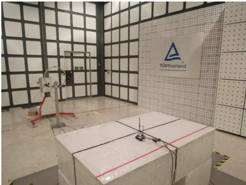
Photograph 5: Set-up for Spurious Emissions (Back View 3)- RFA-02-5-C7H1-ANT
