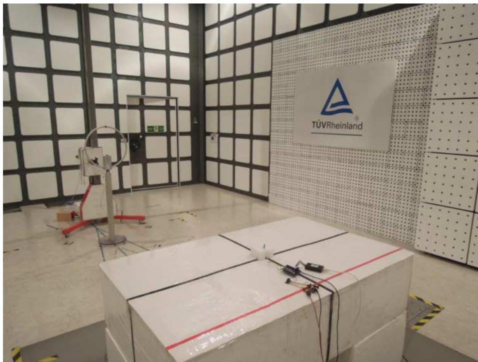
Photograph 17: Set-up for Spurious Emissions (Back View 3)- RFPCA381013IMAB701-ANT
