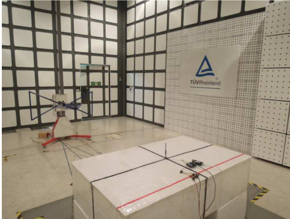
Photograph 3: Set-up for Spurious Emissions (Front View 2)- RFA-02-5-C7H1-ANT
