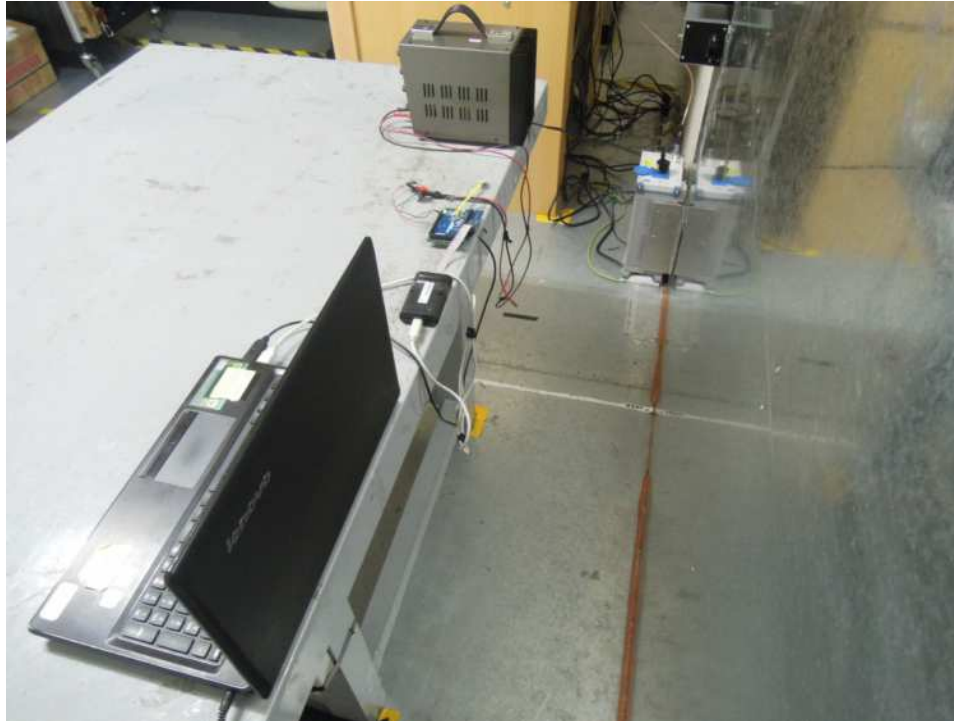
Photograph 36: Set-up for Mains Conducted testing (Back View)
