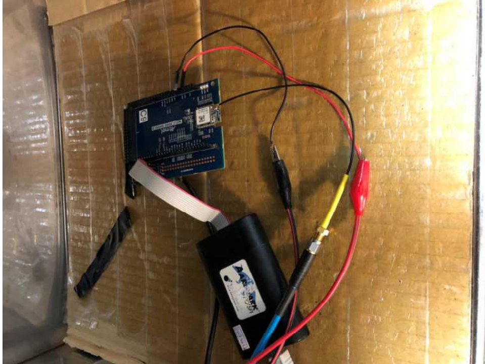
Photograph 35: Set-up for Mains Conducted testing (Front View)
