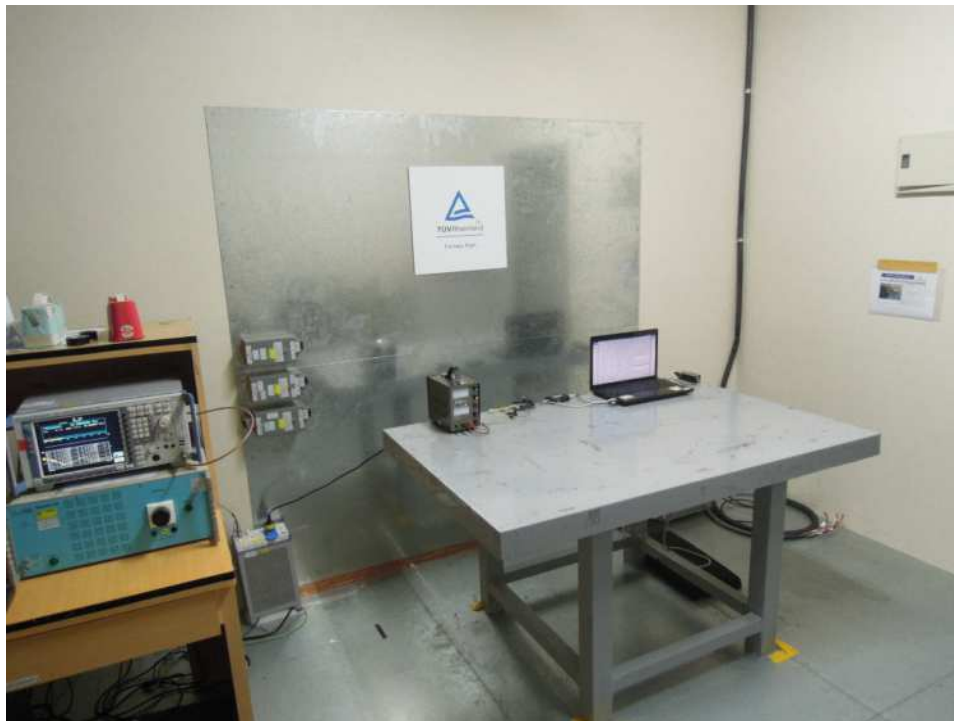
Photograph 35: Set-up for Mains Conducted testing (Front View)
