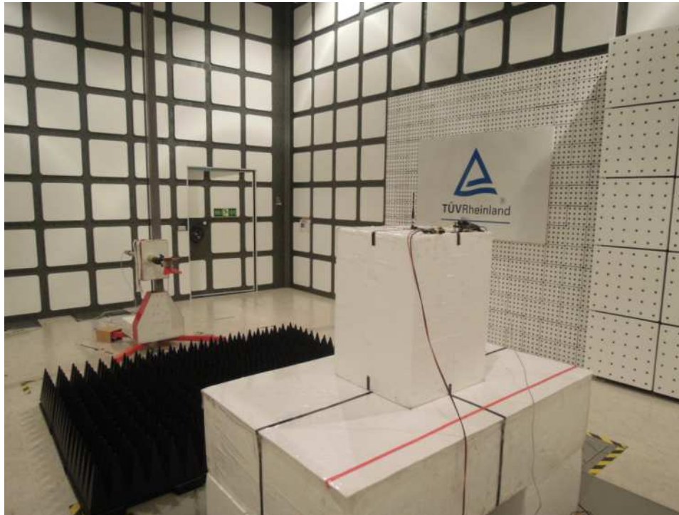
Photograph 5: Set-up for Spurious Emissions (Back View 3)- RFA-02-5-C7H1-ANT
