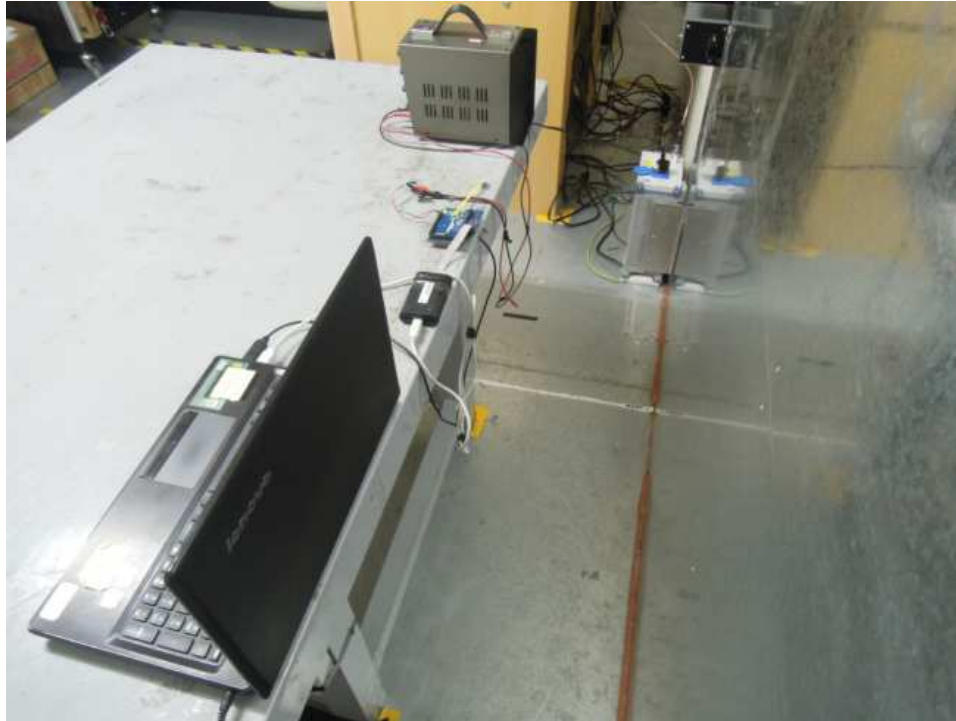
Photograph 36: Set-up for Mains Conducted testing (Back View)
