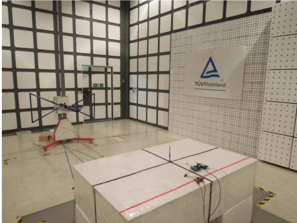
Photograph 3: Set-up for Spurious Emissions (Front View 2)- RFA-02-5-C7H1-ANT
