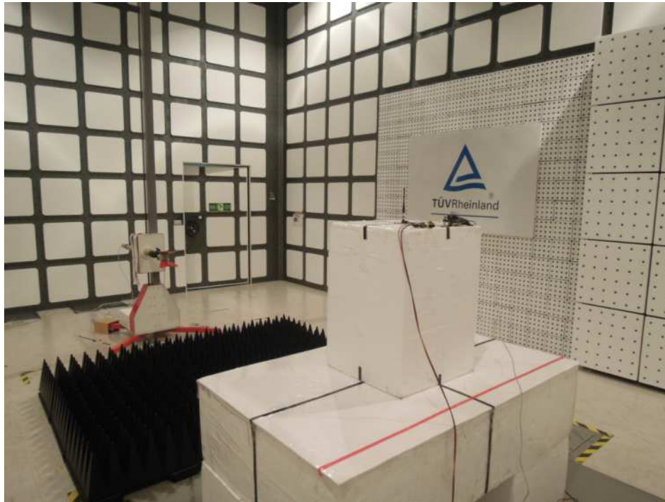
Photograph 5: Set-up for Spurious Emissions (Back View 3)- RFA-02-5-C7H1-ANT
