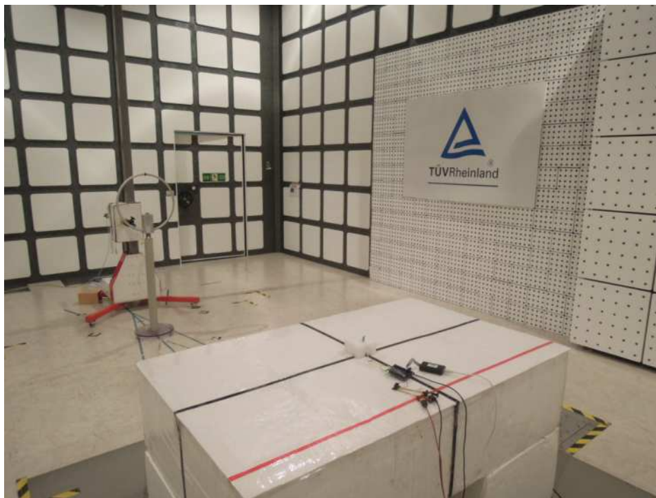
Photograph 17: Set-up for Spurious Emissions (Back View 3)- RFPCA381013IMAB701-ANT
