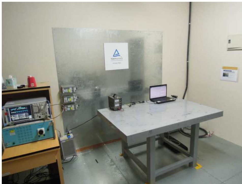
Photograph 21: Set-up for Mains Conducted testing (Front View)
