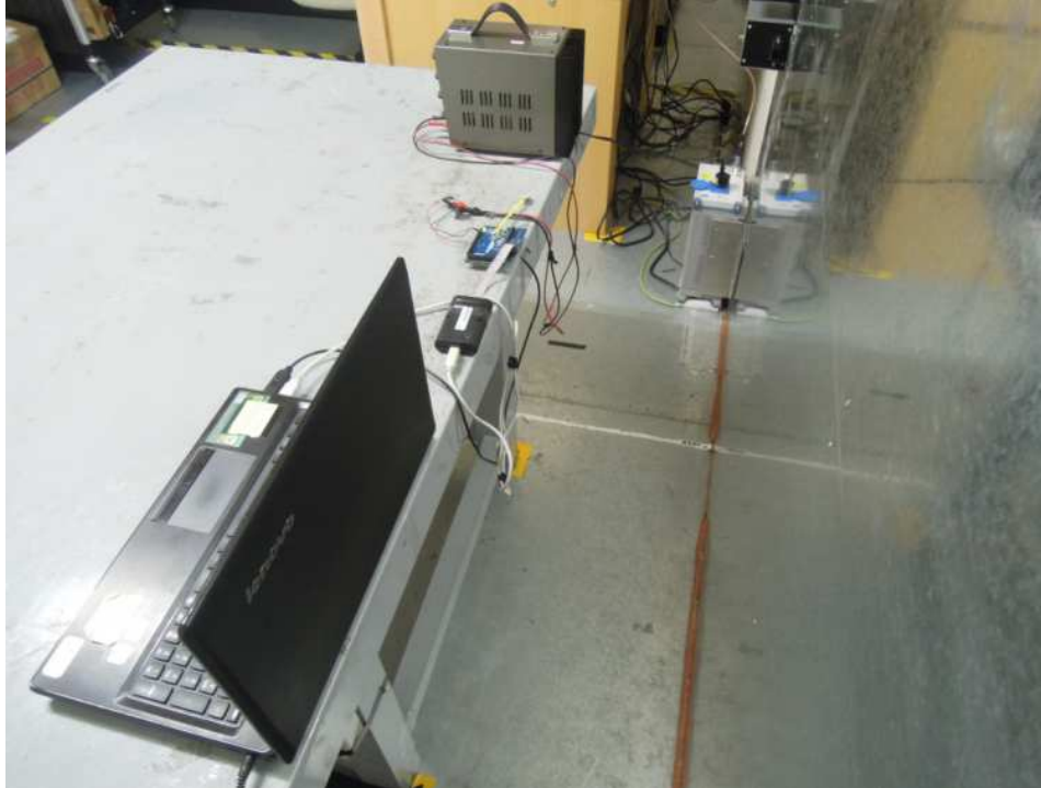
Photograph 22: Set-up for Mains Conducted testing (Back View)
