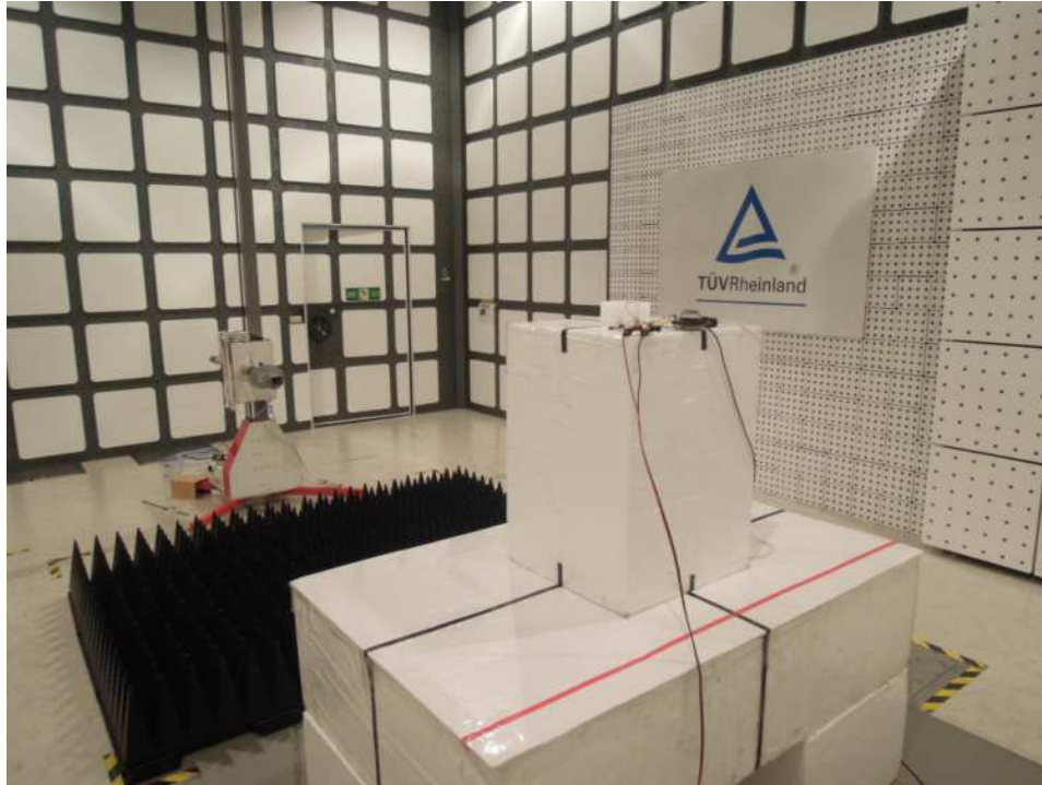
Photograph 13: Set-up for Spurious Emissions (Front View 1)- RFPCA381013IMAB701-ANT
