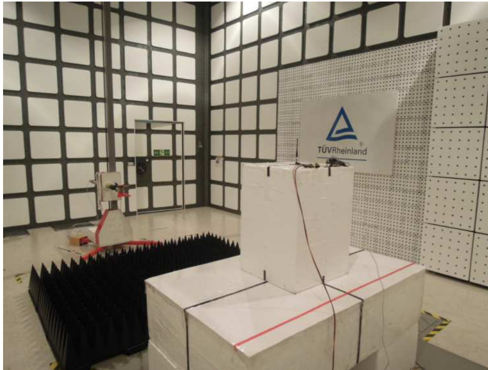
Photograph 5: Set-up for Spurious Emissions (Back View 3)- RFA-02-5-C7H1-ANT
