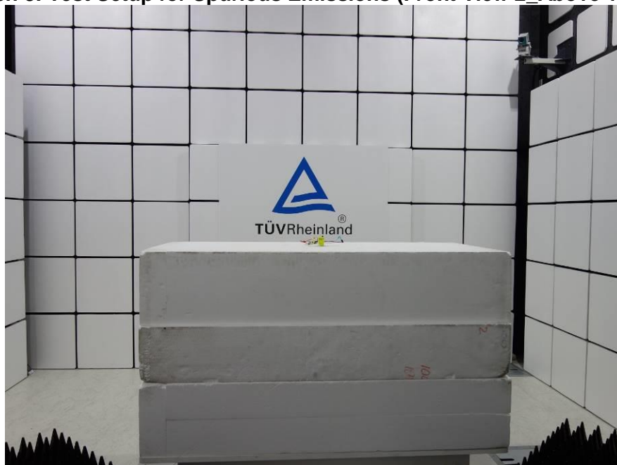
Photograph 8: Test Setup for Spurious Emissions (Front View 2_Above 1GHz)
