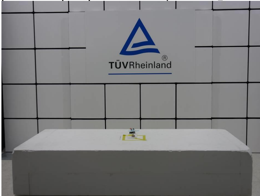
Photograph 2: Test Setup for Spurious Emissions (Front View 2_Above 1GHz)
