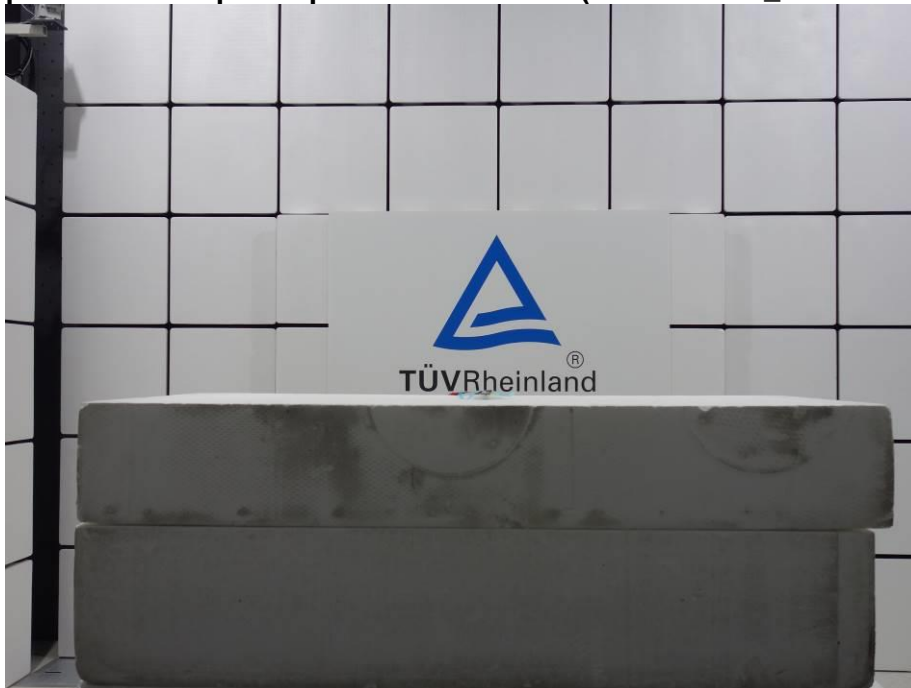
Photograph 2: Test Setup for Spurious Emissions (Front View 2_Above 1GHz)
