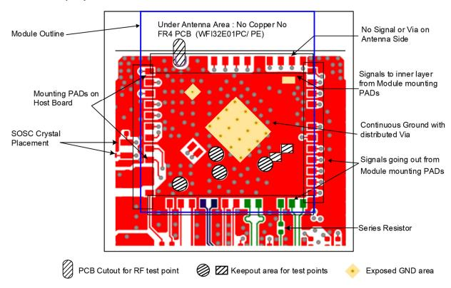
The top layer (underneath the module) of the host PCB must be ground with as many GND vias as possible.
