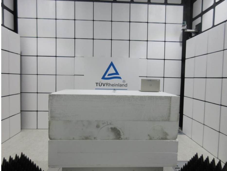
Photograph 19: Set-up for Spurious Emissions (Front View, #207)
