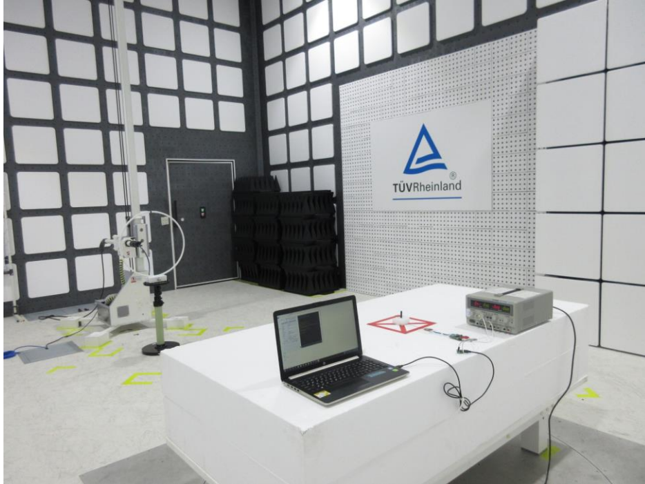
Photograph 5: Set-up for Spurious Emissions (Back View 3, #5)
