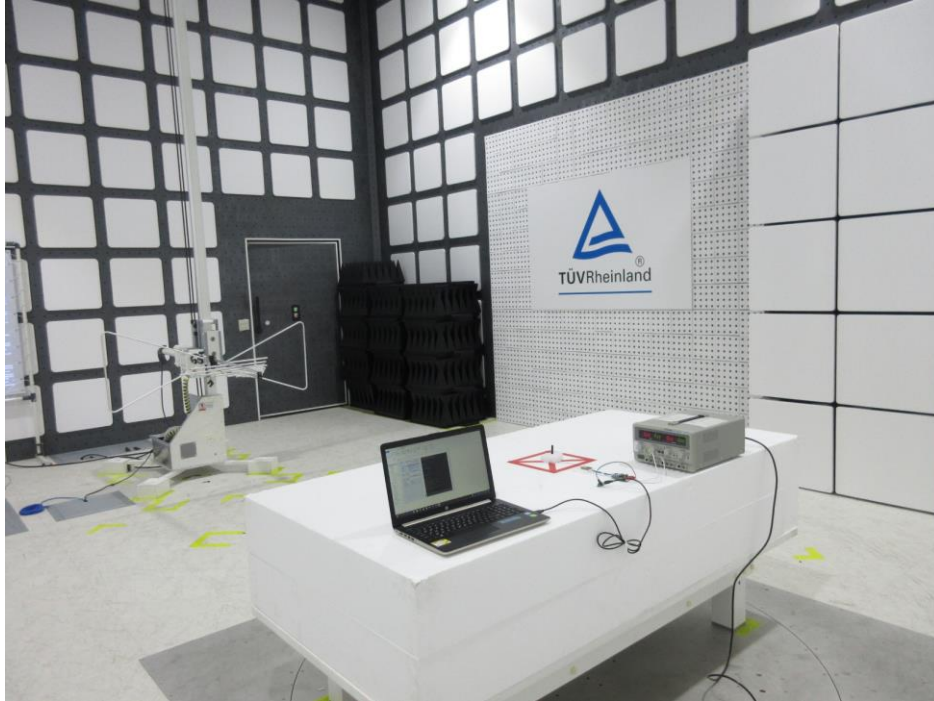
Photograph 3: Set-up for Spurious Emissions (Back View 1, #5)
