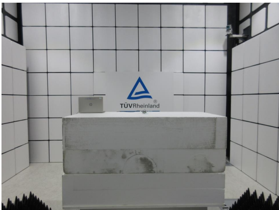
Photograph 16: Set-up for Spurious Emissions (Front View, #64)
