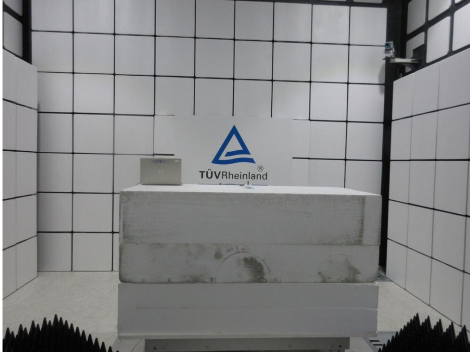
Photograph 13: Set-up for Spurious Emissions (Front View, #61)
