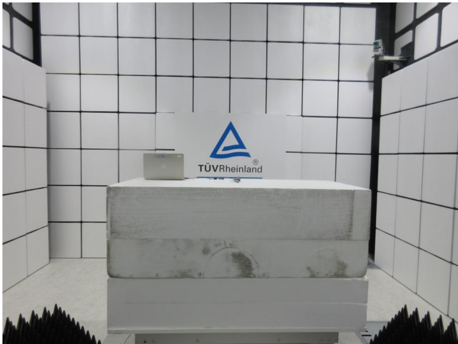
Photograph 22: Set-up for Spurious Emissions (Front View, #221)
