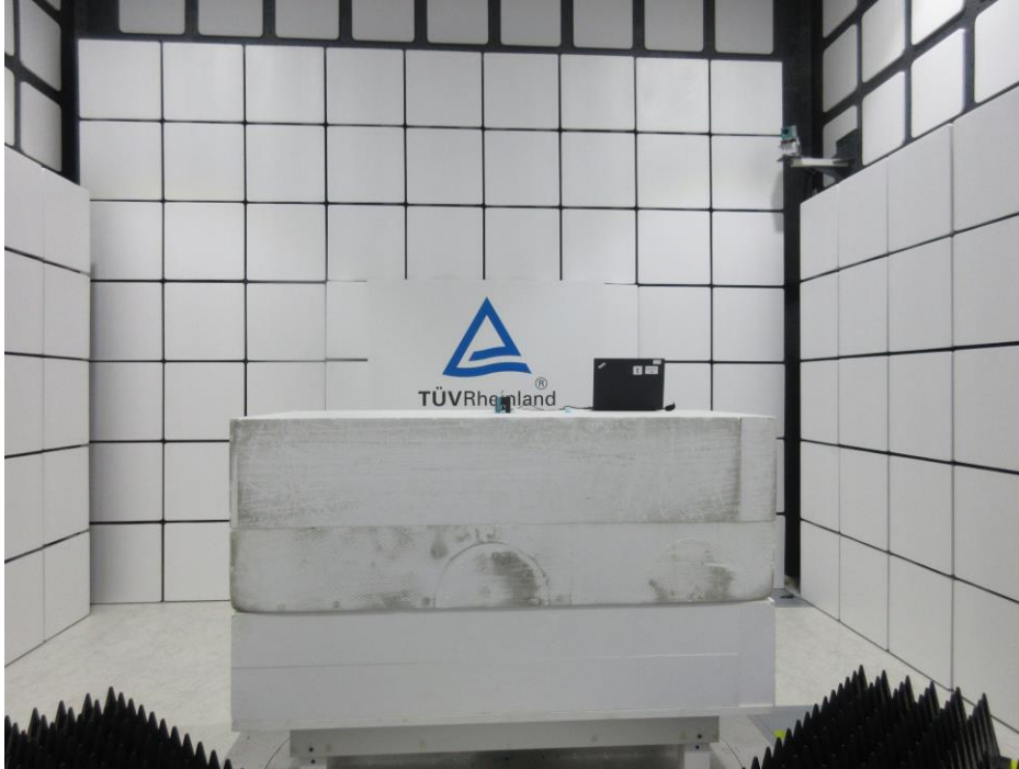
Photograph 31: Set-up for Spurious Emissions (Front View, #214)
